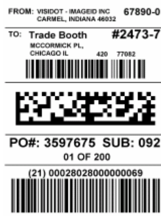
Figure 9: EAN-128 pallet label with a 2D Data Matrix
